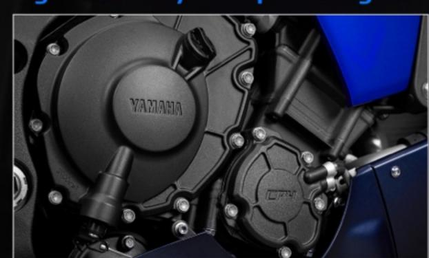
A key feature of the R1's EU5 998cc engine is the crossplane crankshaft with its uneven 270°-180°-90°-180° firing sequence that delivers strong, linear torque. Featuring a high-efficiency intake system along with specially designed finger-follower rocker arms, this race- developed engine delivers remarkable high rpm performance
