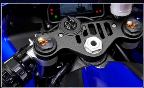
Control is everything when you're on the road or track, and the Engine Brake Management (EBM) system allows you to adjust engine braking force. Using data from various sensors, the EBM adjusts throttle opening, ignition timing and fuel injection volume to give you a choice of three engine braking modes to suit different riding situations.
