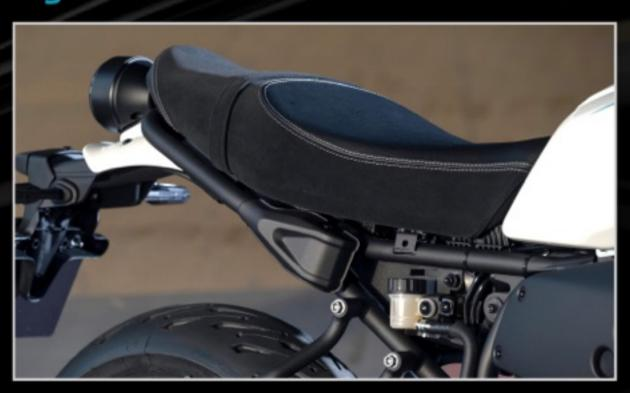
For easy manoeuvrability and sharp agility, the XSR700 runs with a slim, light steel backbone frame that is easily customisable due to its two piece subframe. Combined with its compact wheelbase and easy natured suspension system, this strong and light chassis gives a responsive and engaging ride.
