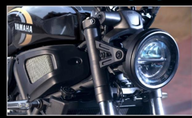
The XSR700 is fitted with a heritage inspired round LED headlight with a split projector and a semi-circular position lamp. The LED tail light features a classically shaped round form, and the compact LED indicators are more subtly shaped, whilst providing outstanding visibility.
