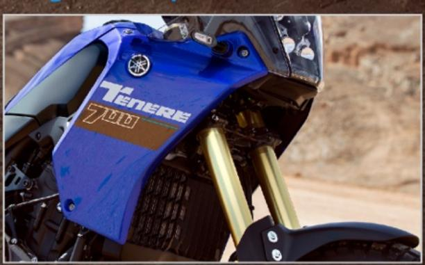
Check out the race-bred front suspension, and it's clear that this lightweight adventure bike is built to take on the most hostile terrain! Equipped with flex-resistant 43 mm tubes and offering 210 mm of front wheel movement that gives a smooth ride with lightweight steering, these adjustable upside-down forks can handle whatever you may encounter on your adventures!
