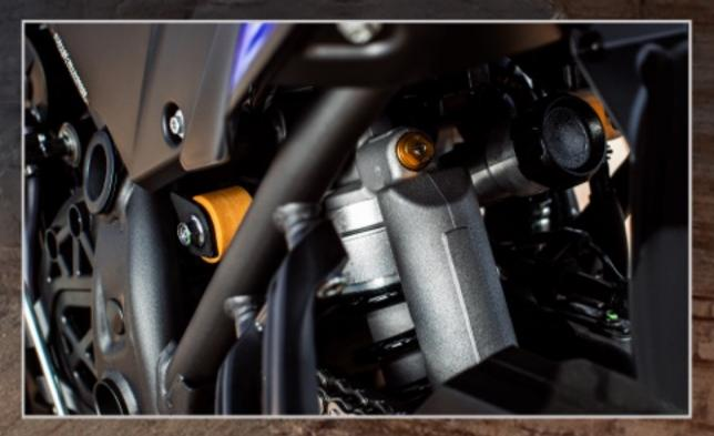
The sophisticated rear suspension is designed to give you a smooth and stable ride in a variety of conditions on the dirt or highway - whether you're riding solo or carrying a passenger and luggage. Offering 200mm of wheel movement, this rally-bred system features a convenient, remote adjuster, enabling you to adjust the settings while you're on the go.
